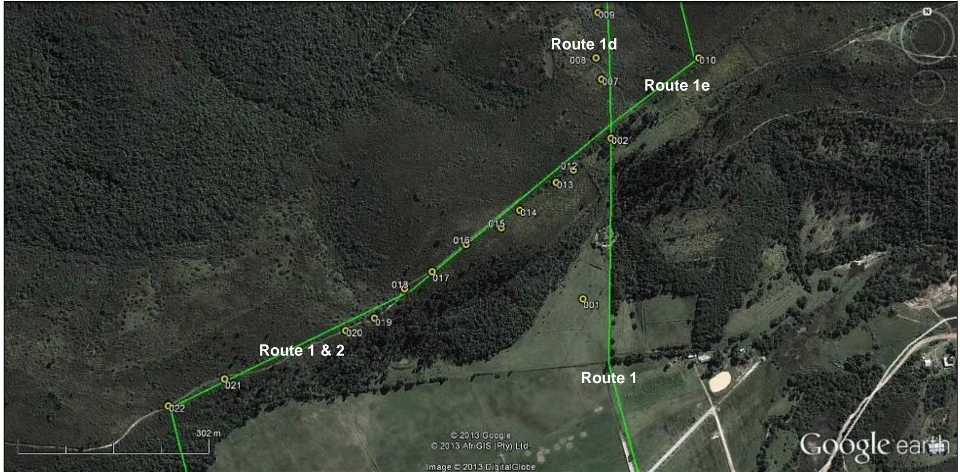
**Figure 16.** Google Earth™ aerial image showing the proposed 66kV powerline Routes 1 & 2, Route 1, Route 1d and 1d (green lines) between waypoint 022 and 009. The numbered yellow circle icons are the waypoints from the 2013 survey.
