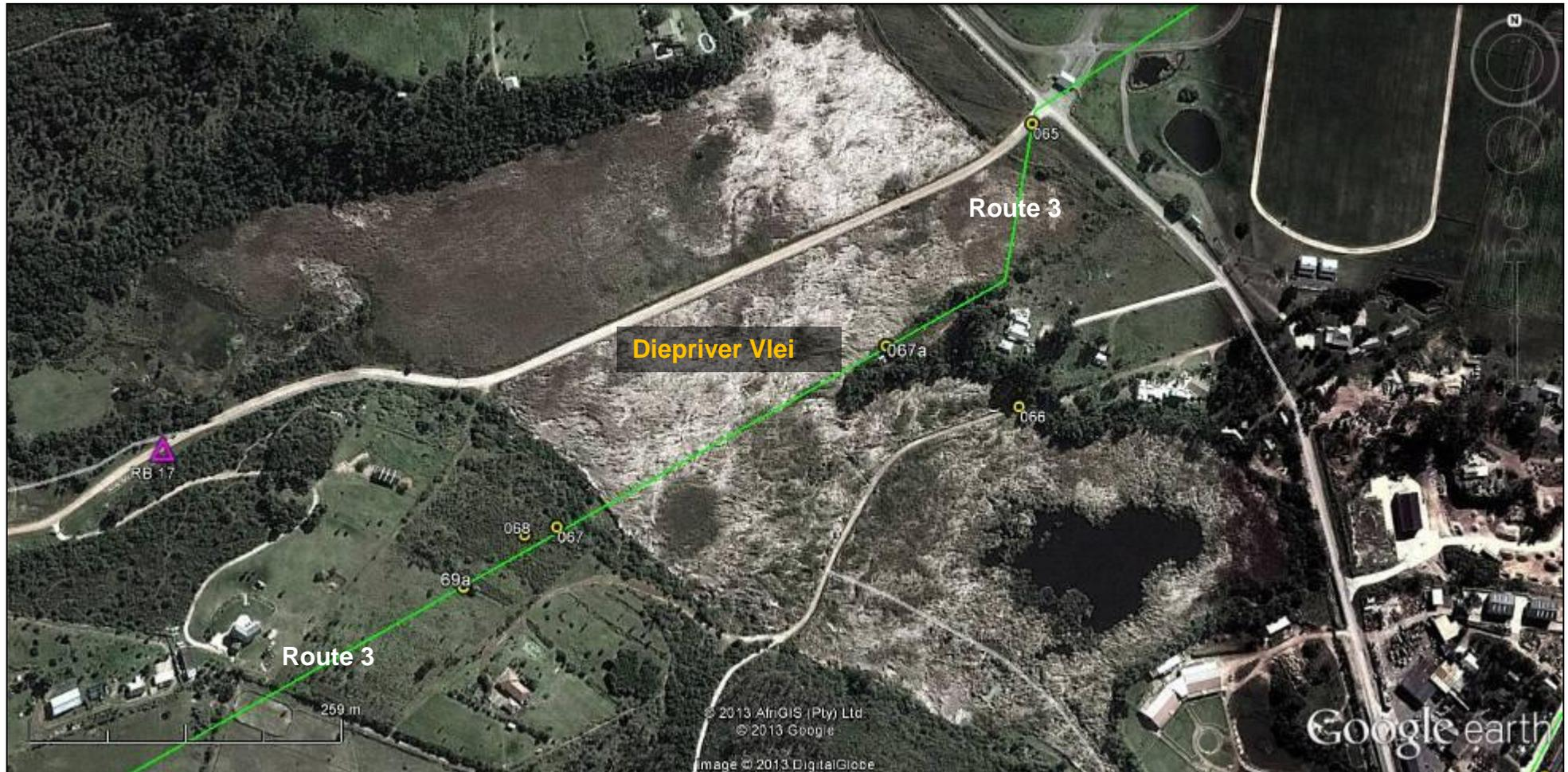
**Figure 10.** Google Earth™ aerial image showing the proposed 66kV powerline Route 3 (green lines) between placemark 69a to waypoint 065. The numbered yellow circle icons are the waypoints from the 2013 survey whereas the numbered purple triangle icons are from McDonald's (2007) survey. The numbered icons 69a and 67b are placemark points, i.e. not field samples but used to designate key features in the landscape.
