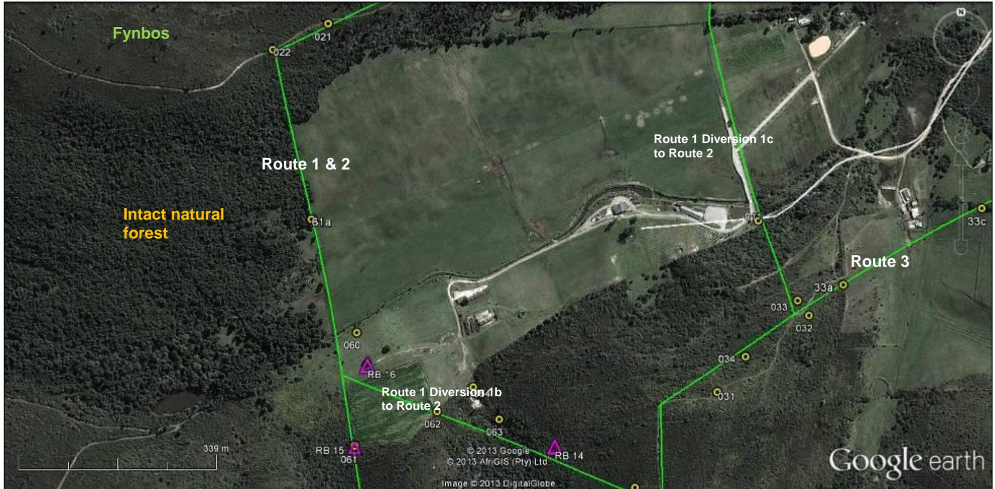
**Figure 15.** Google Earth™ aerial image showing the proposed 66kV powerline Route 1 & 2, Route Divesrion1b and 1c to Route 2 and Route 3 (green lines) between waypoint 061 and 022 and. The numbered yellow circle icons are the waypoints from the 2013 survey. The numbered purple numbered icons with the 'RB' prefix are McDonald's (2007) sample waypoints.
