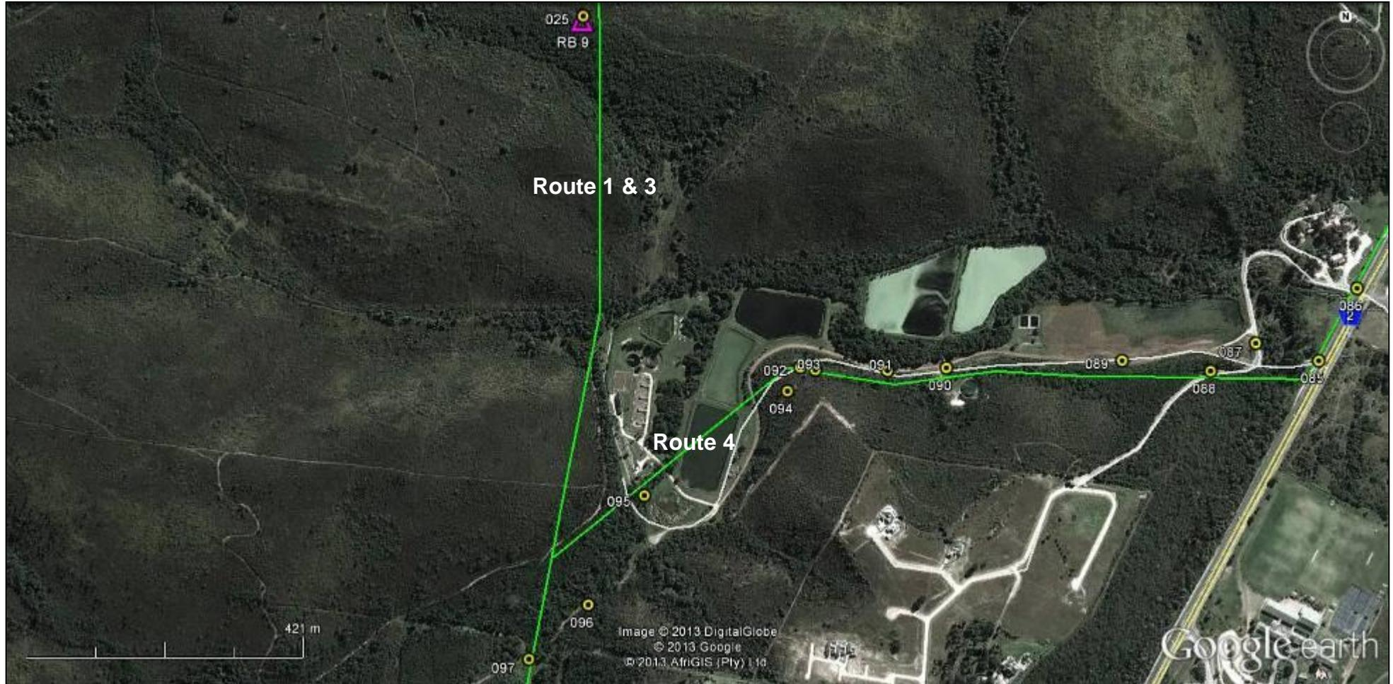
**Figure 7.** Google Earth™ aerial image showing the proposed 66kV powerline routes 1, 3 & 4 (green lines) between waypoints 097 to 025. The numbered yellow circle icons are the waypoints from the 2013 survey whereas the numbered purple triangle icons are from McDonalds 2007 survey.
