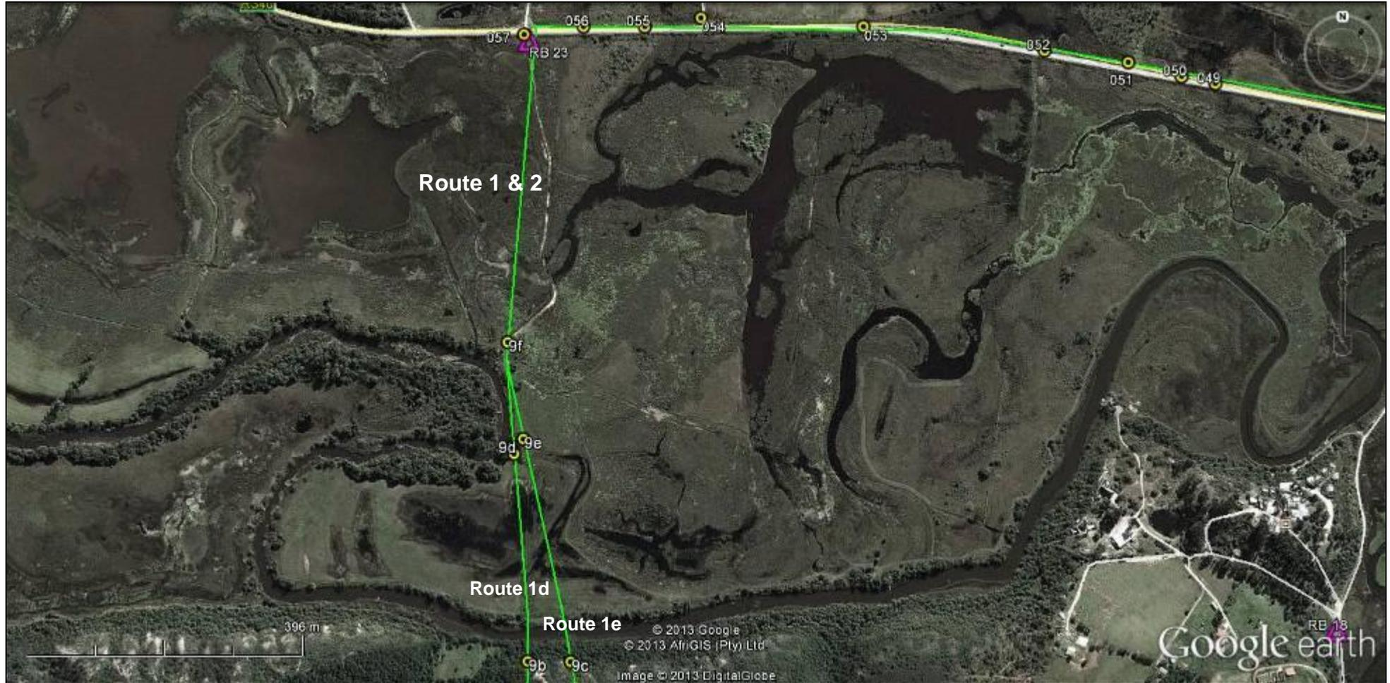
**Figure 18.** Google Earth™ aerial image showing the proposed 66kV powerline Route 1 & 2 and Routes 1d & 1e (green lines) between waypoint 013 and placemarks 9b & 9c. The numbered yellow circle icons are the waypoints from the 2013 survey.
