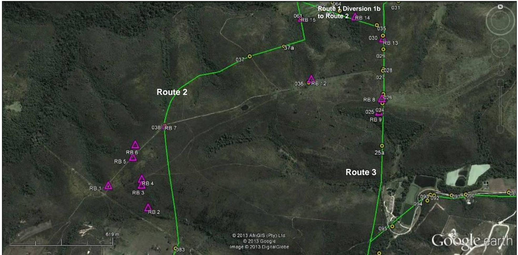
**Figure 14.** Google Earth™ aerial image showing the proposed 66kV powerline Route 2 and Route 3 (green lines) between waypoint 083 and 061. The numbered yellow circle icons are the waypoints from the 2013 survey. The numbered purple numbered icons with the 'RB' prefix are McDonald's (2007) sample waypoints.
