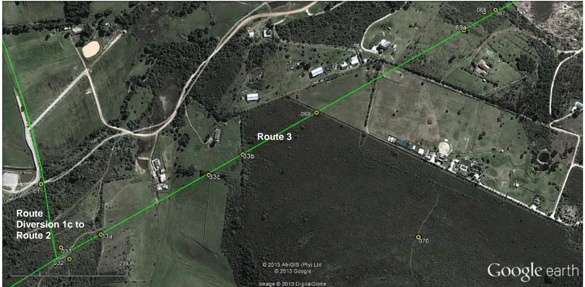
**Figure 9.** Google Earth™ aerial image showing the proposed 66kV powerline route 3 (green lines) between waypoints 033 to 067. The numbered yellow circle icons are the waypoints from the 2013 survey. The numbered icons 33a and 33b are placemark points, i.e. not field samples but used to designate key features in the landscape.
