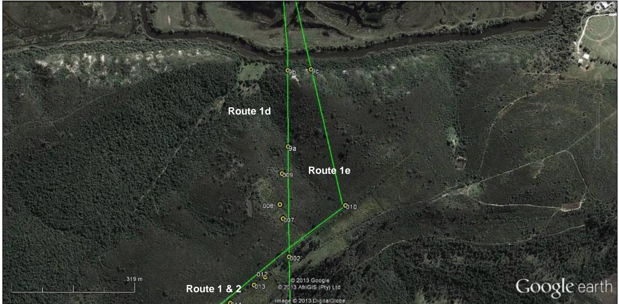
**Figure 17.** Google Earth™ aerial image showing the proposed 66kV powerline Route 1 & 2 and Route 1d & 1e (green lines) between waypoint 013 and placemarks 9b & 9c. The numbered yellow circle icons are the waypoints from the 2013 survey.
