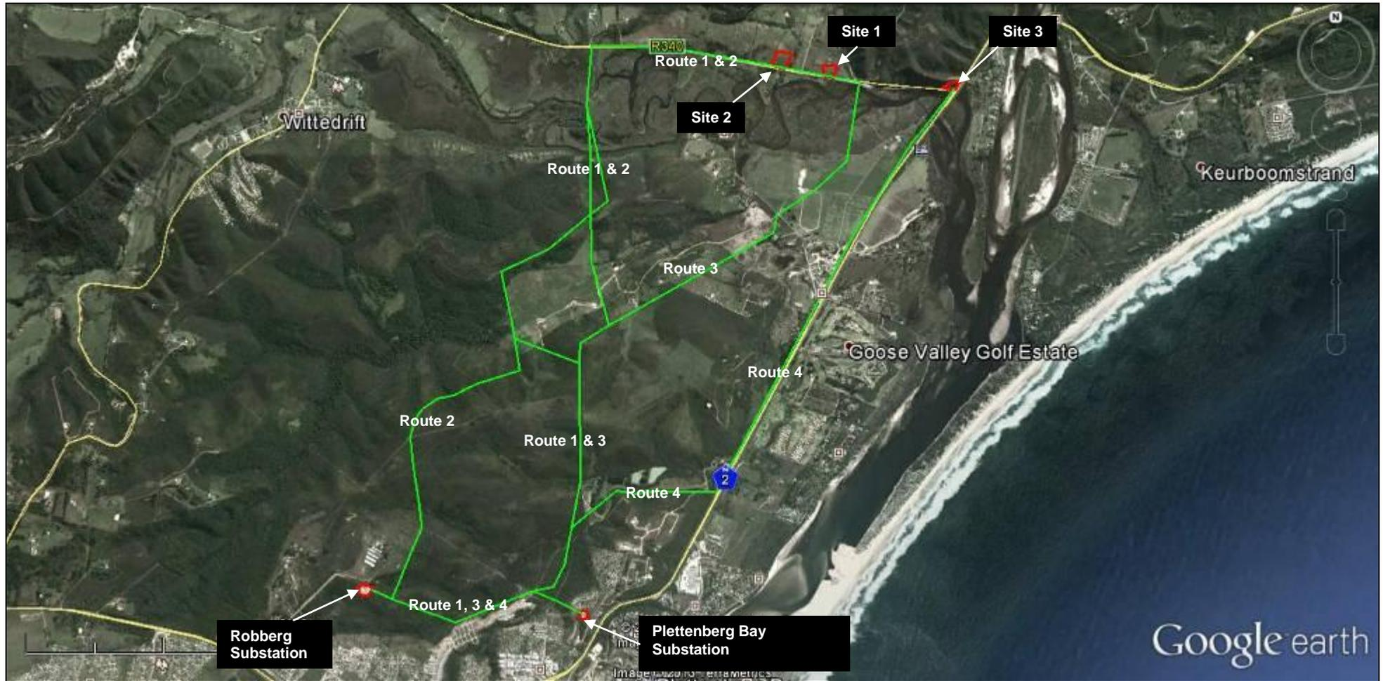
**Figure 2.** Google Earth™ aerial image showing the proposed 66kV powerline routes 1, 2, 3 & 4 (green lines) and substation sites 1, 2 & 3 (red boundary lines).
